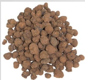
broken expanded clay
